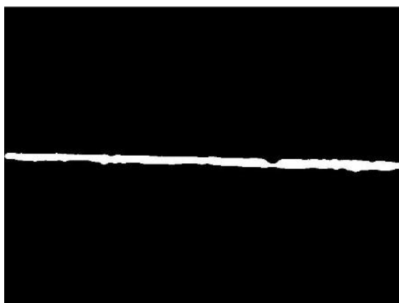
Figure 8: Segmentation result of weld area.
